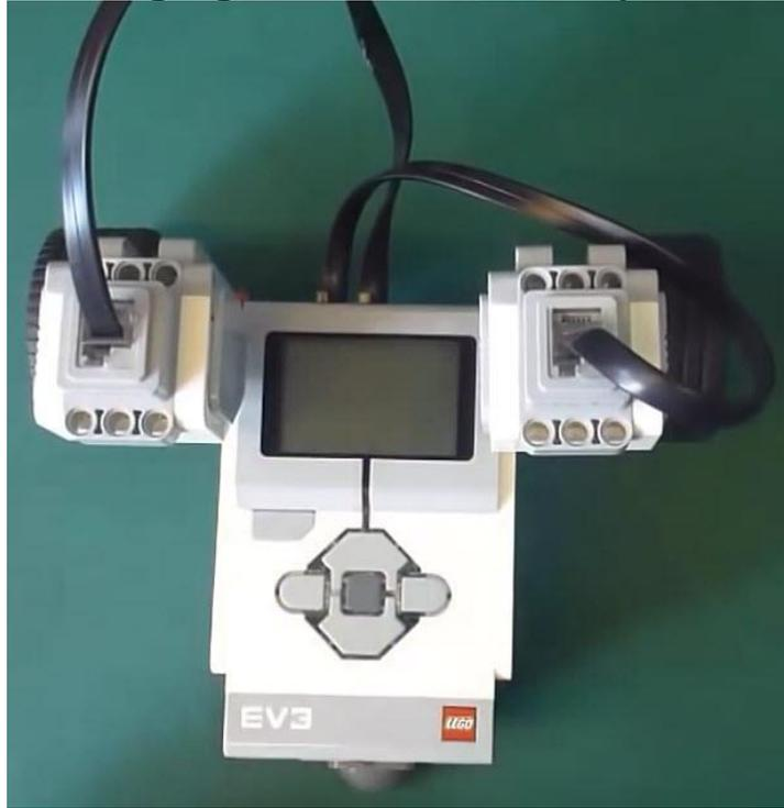
Botticelli is a really nice Robot, but we found that it had problems going backwards on some carpets that had ridges, so to fix this we will redesign our Robot by adding a back wheel and changing the motors. We will name our new Robot LucyBot.
